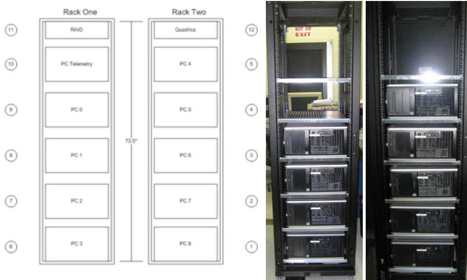
Figure 3: Left: Rack layout design. Right: Partially populated computer racks in our lab.
