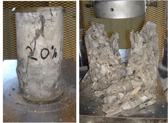
Fig. 6. Compressive strength testing for 20% RCON cylinders
