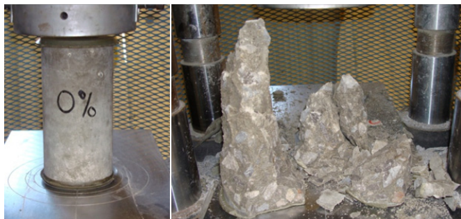
Fig. 5. Compressive strength testing for a 0% RCON cylinders
