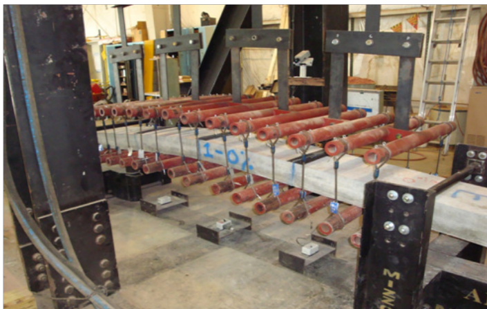
Fig. 2. Typical sample being tested in loading tree
