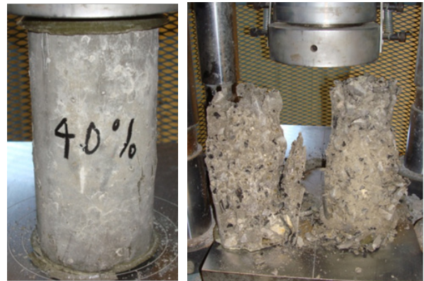
Fig. 7. Compressive strength testing for 40% RCON cylinders
