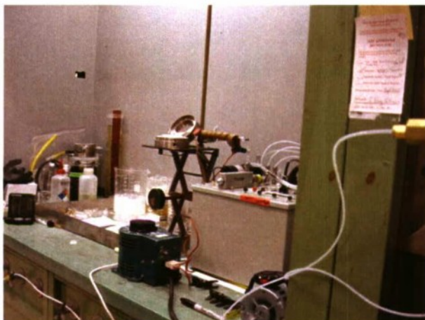
Figure 13. MINICAMS near real-time monitoring system, single vapor cup.
