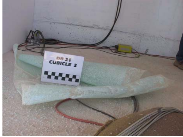
(b) Glass debris on floor near back of cubicle.
