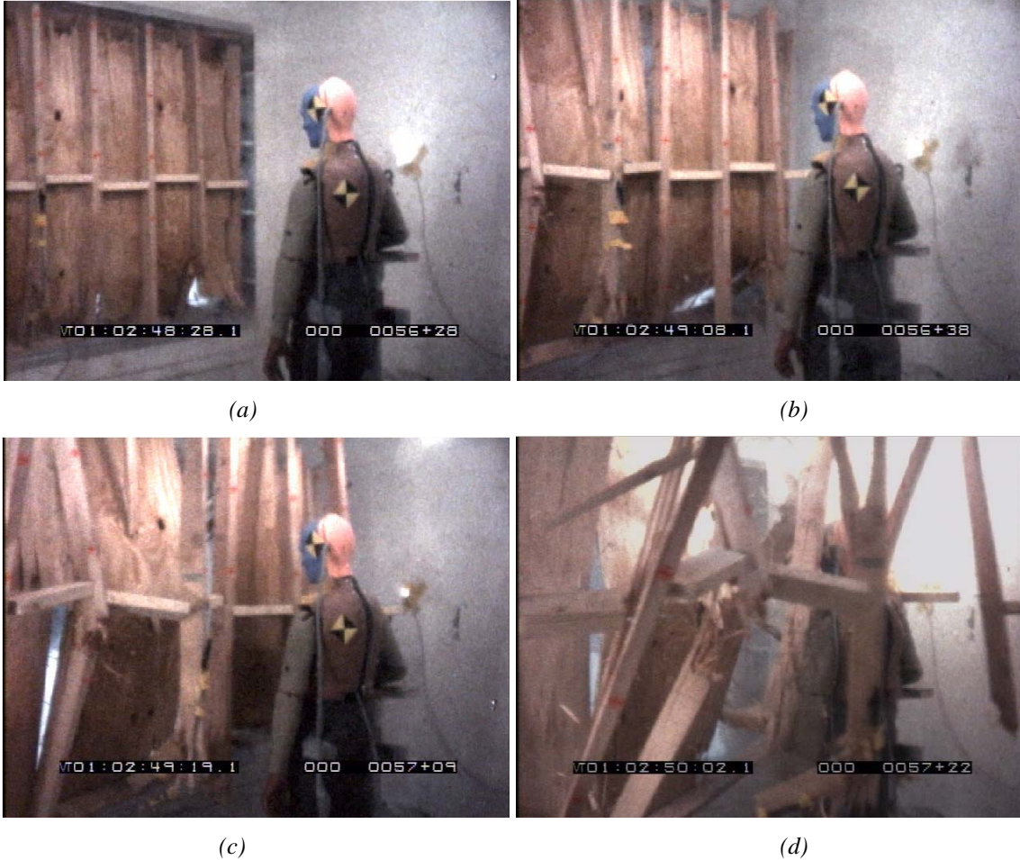
Figure 18. Snapshots of standing ATD impacted by wood debris.
