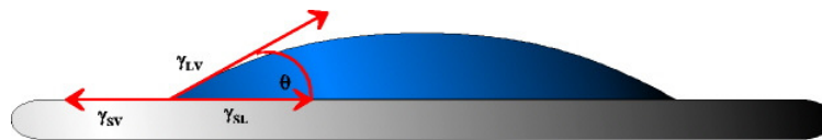
Figure 3: Contact angle measurement for evaluation of wettability
