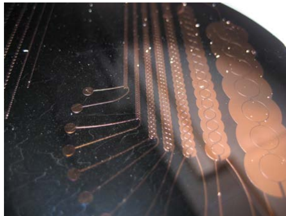
Figure 12: Silicon wafer with copper pads of different size, to be used with small volumes of LMP and paraffin
