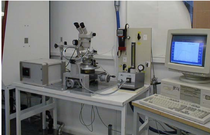
Figure 20: Lab setup for formic acid vapor soldering in controlled atmosphere.
