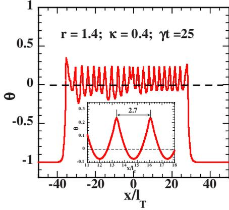
FIG. 5. (Color online) Profile of the  $J_c$  ripples ( $r=1.4$ ,  $\kappa_0=0.4$ ) at a certain moment of time,  $\gamma t=25$ . The inset shows a magnified view of the same profile. The periodicity of the  $J_c$  ripple is  $\approx 2.7l_T$ . The peak temperature is  $\theta_p \approx 0.24-0.26$  in agreement with the exact value  $1-r^{-1}$ , Eq. (51).
