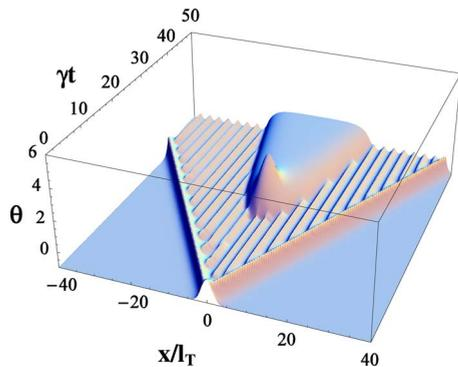
FIG. 7. (Color online) Tristable operation which corresponds to  $\kappa_0=0.4$ ,  $r=1.4$ , and  $\theta_0=-1$ . The initial profile evolves into  $J_c$  ripples. A heater, Eq. (54), is switched on at  $\gamma t=20$  and switched off at  $\gamma t=25$ . It triggers the transition to the normal state. The evolution of the system depicted in the figure corresponds to  $b=1.5$ ,  $\delta_1=1.4$ .
