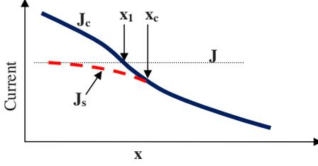
FIG. 2. (Color online) The solid line is a sketch of the temperature-dependent critical current density  $J_c$ . Temperature increases from left to right. The dashed line  $J_s$  is the current density that flows through the superconductor. The dotted line is the constant total current density. The point  $x_c$  demarcates the boundary between the subcritical  $E_s=0$  and critical  $E_s>0$  sections.
