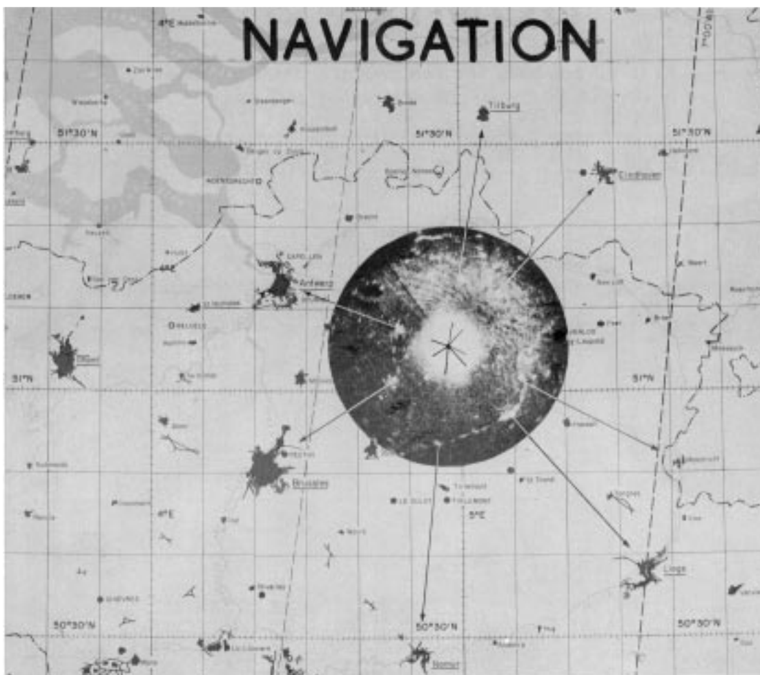
H2X was a self-contained radar device whose beam scanned the ground below the aircraft within a radius of up to 50 miles and provided a radar map of the terrain on its cathode-ray scope. The center of the scope represented the position of the aircraft, and the bright spots were presumed to be cities or landmarks.
