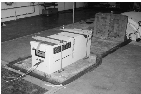
Figure 3. Fuel cell system FC-250 undergoing vibration testing.
