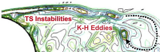
Fig. 6. Snapshot of the spanwise vorticity contours (max. -11, min. -16, incr. 0.5 and max. 25, min. -25, incr. 2.5) showing the TS instabilities and K-H eddies within the free-shear layer of the yaw circular cylinder ( \alpha = 45^\circ ).
