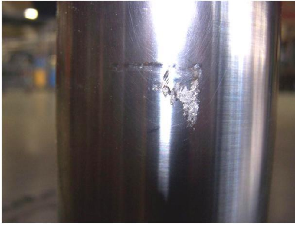
Figure 13 – Damage on probe post test.
