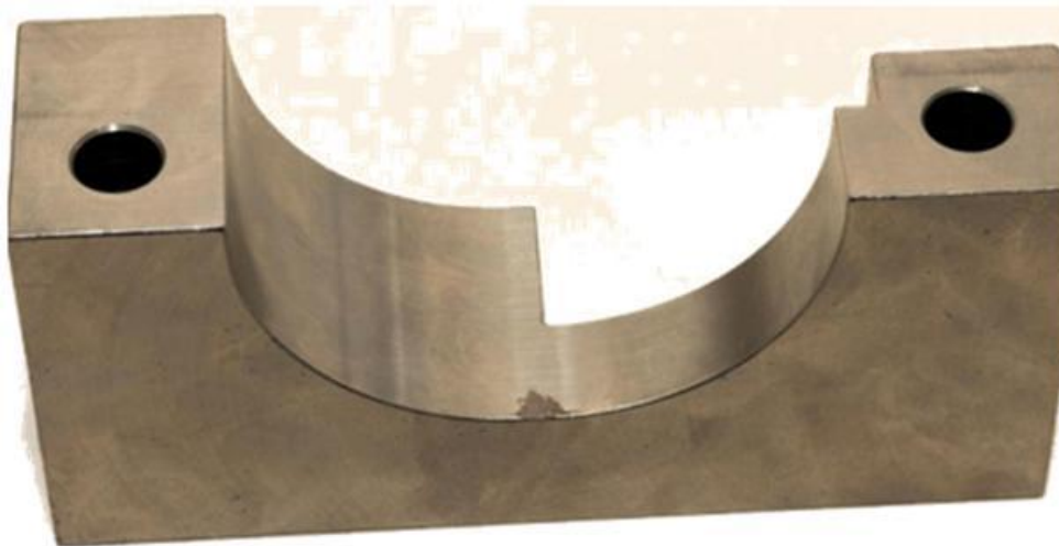
Figure 12 – Damage on RSD simulator fixture post test
