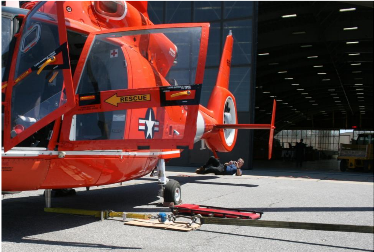
Figure 18 – Static Load Test Setup, 270 Deg. (Port) Load Case
