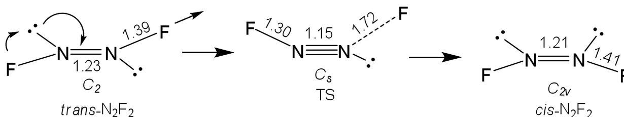
It has a structure similar to that of the  $\text{N}_2\text{F}^+$  cation with a significantly shortened N-F bond of 1.30 Å, a very short N-N bond of 1.15 Å, and an F-N-N angle of  $170^\circ$ . The second N-F bond is elongated to 1.72 Å. This transition state has an imaginary frequency of  $883i \text{ cm}^{-1}$  and lies 68.7 kcal/mol above the ground state. Thus, contrary to our previous speculation,<sup>9</sup> the
