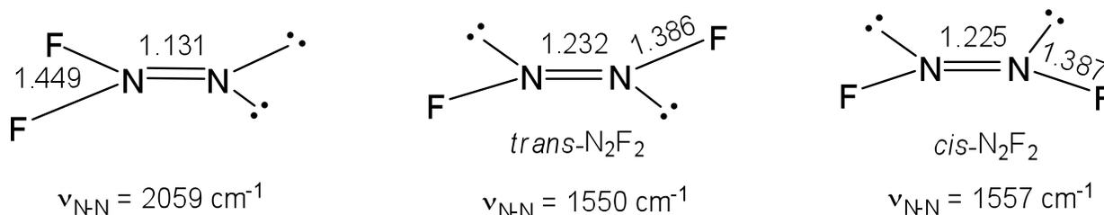
Similarly, the N-N stretching frequency is increased by about  $500 \text{ cm}^{-1}$ , while the  $\text{NF}_2$  stretching frequencies are decreased by an average of about  $300 \text{ cm}^{-1}$ , indicating that in  $\text{F}_2\text{N}=\text{N}$ , strong contributions from the following resonance structures must be invoked to describe its bonding appropriately.
