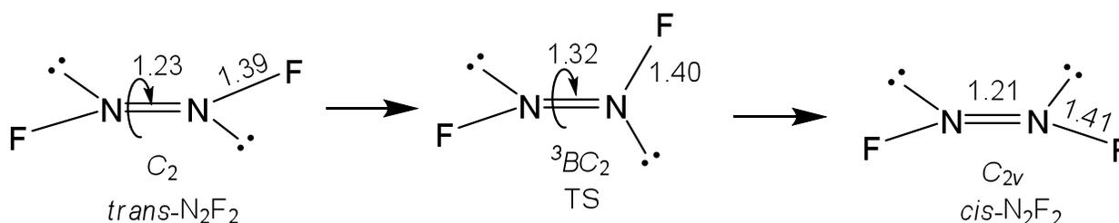
The calculated  ${}^3B C_2$  minimum energy structure with a dihedral F-N-N-F angle of  $89.8^\circ$  (Table 6) lies 59.6 kcal/mol above the *cis*-isomer at 0 K. This represents the lower limit to the isomerization barrier on the singlet surface. The value of  $\sim 60$  kcal/mol for rotation about the N=N bond is consistent with the value expected for the C=C  $\pi$ -bond.<sup>71</sup>
