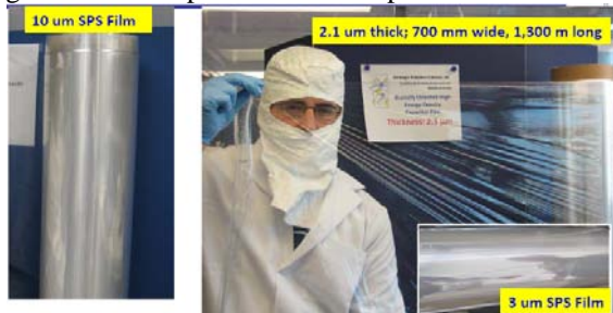
Figure 4. High quality ultra-thin SPS capacitor film produced by melt-extrusion and biaxial orientation.
