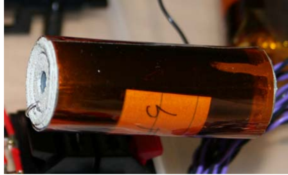
Figure 2. Picture of pre-packaged capacitor cores after winding the \text{SiO}_2 coated metalized polyimide electrodes into a cylindrical shape and end spray.
