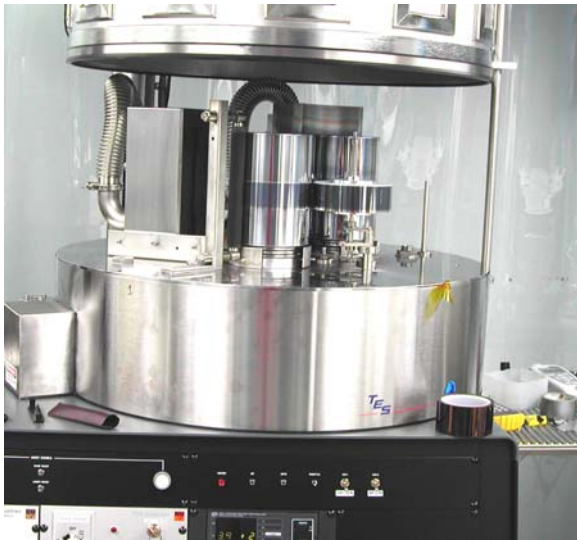
Figure 1. Picture of the custom built web coating system used to deposit the dielectric on the metalized film.
