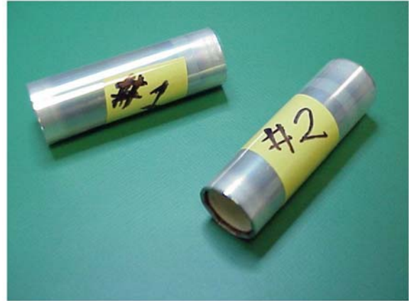
Figure 5. Picture of pre-packaged capacitor cores after winding the SiO 2 coated metalized polyester electrodes.
