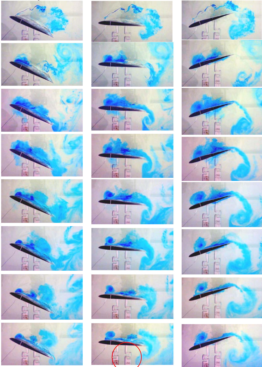
Figure 48. 8 periods of trapezoidal pitch: dye injection at phases a (left column), b (middle column) and c (right column); time from motion onset is from top to bottom. Top row is first period, second row is second period, and so forth, down to the 8 th period. Double trailing vortex system is circled.
