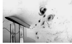
Figure 57. Dye injection for 4 different starting phases of pure-pitch motion; k = 3.93 , pivot about x/c = 0.25 , Re = 10K , dye injected at trailing edge; periods of oscillation as marked, from start of motion.
