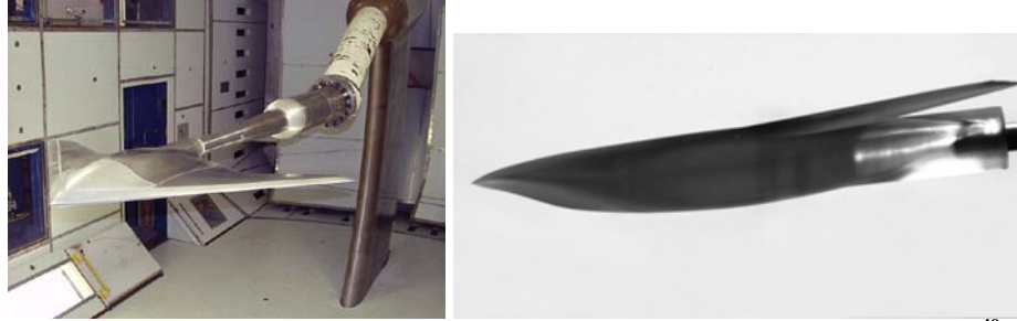
Figure 4. The 1303 UCAV configuration: 5'-span model installed in QinetiQ 5m wind tunnel 49 , and 3D-printed (plastic) installed in water tunnel test section 50 .
