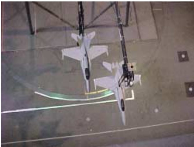
Fig. 1.3 FA-18 FORMATION STUDIES IN WIND TUNNEL
