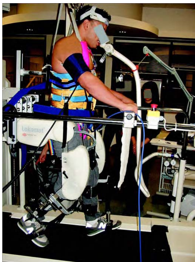
Figure 2. Metabolic testing in Lokomat (Hocoma AG; Volketswil, Switzerland).
