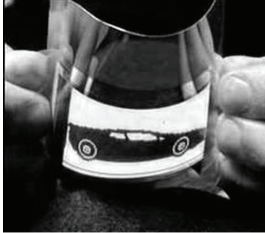
Figure 4-47. Prototype FOLED (Flexible Organic Light Emitting device) technology, using a flexible substrate (Source: Universal Display Corporation, 2007).
