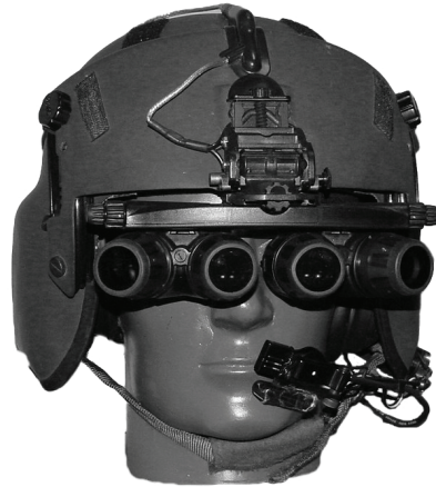
Figure 12-47. Panoramic Night Vision Goggles (PNVG).
