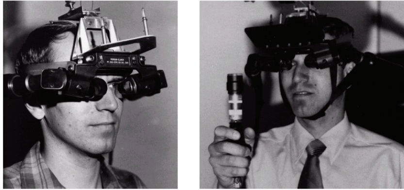
Figure 3-15. Ivan Sutherland's HMD (late 1960's) (Department of Computer Science, University of Utah).
