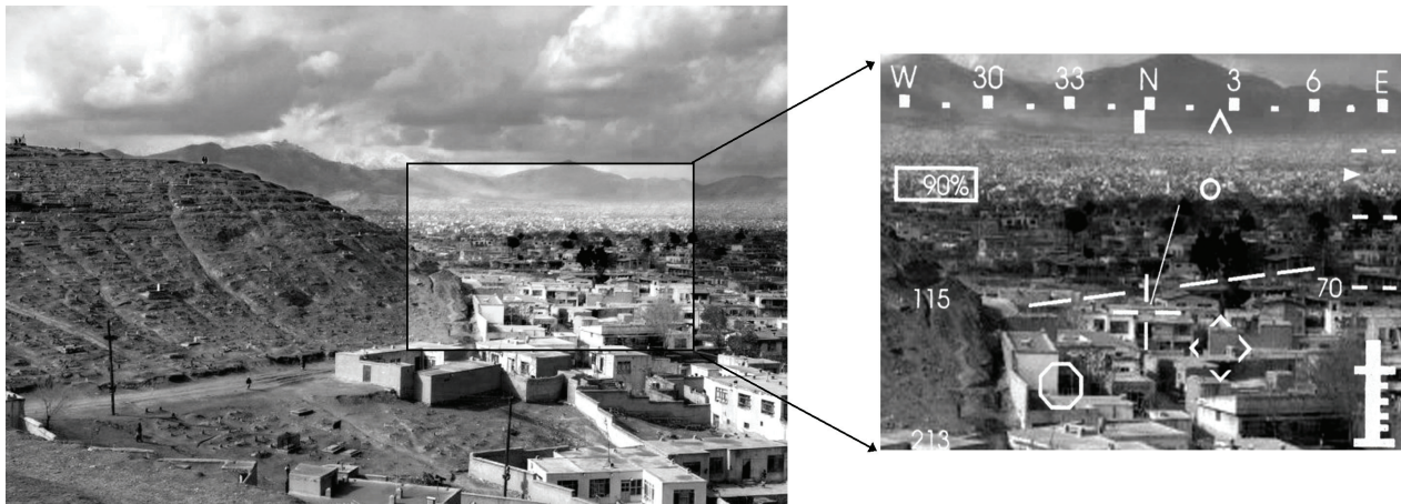
Integrated Helmet and Display Sighting System (IHADSS)
