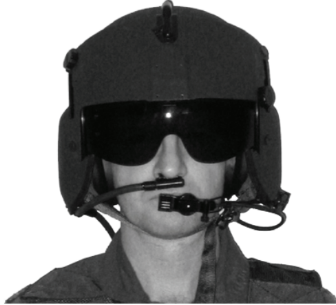
Figure 16-12. PHODS device installed on Gentex HGU-56/P US Army helicopter helmet.
