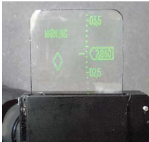
Figure 3-28. View of symbology through Q-Sight (BAE Systems).
