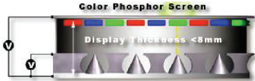
Figure 4-32. Operation of a Field Emission Display (Pixtech, Inc.).
