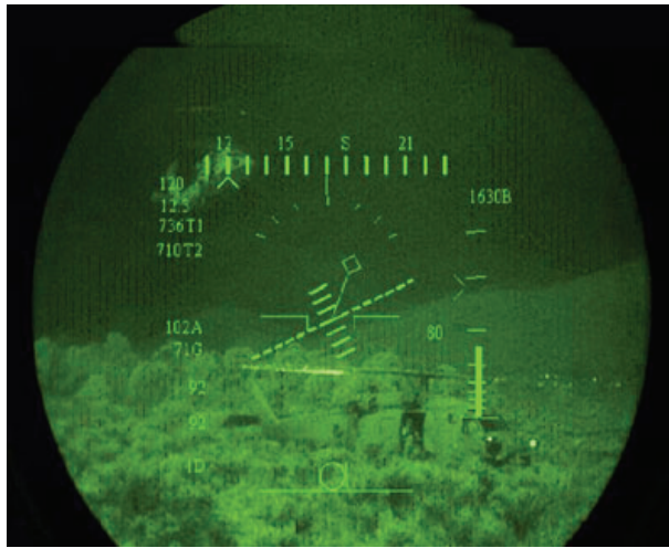
Figure 3-23. Typical ANVIS/HUD-7 imagery: Symbology overlaid on night imagery.
