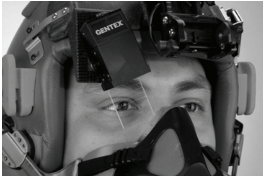
Figure 3-21. Scorpion Helmet Mounted Cueing System (Gentex Corporation),
