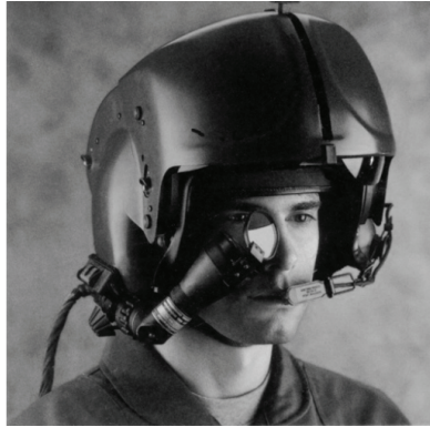
Integrated Helmet and Display Sighting System (IHADSS)
