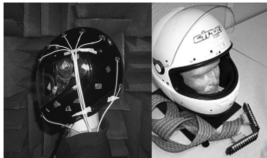
Figure 5-32. Motorcycle helmet with microphone array built at ATI (left) and at ARL (right) for natural hearing restoration research (Courtesy of ATI and U.S. Army Research Laboratory).
