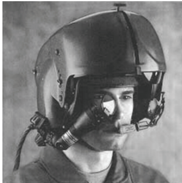
Figure 1-1. A representative HMD, the Integrated Helmet and Display Sighting System (IHADSS), used on the U.S. Army's AH-64 Apache attack helicopter.
