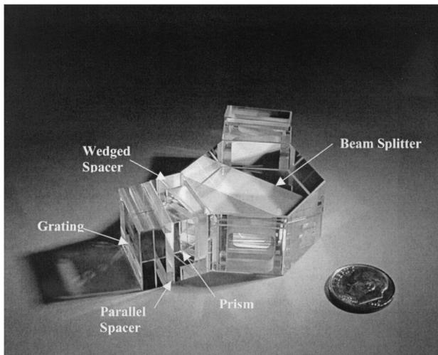
Fig. 2. Monolithic SHS interferometer. The beam splitter (the central hexagonal section) faces are  $20\text{ mm} \times 20\text{ mm}$ . Working outward in each arm the first elements are wedged spacers that mate the beam-splitter faces to the field-widening prisms. Parallel spacers mate the prisms to the gratings.
