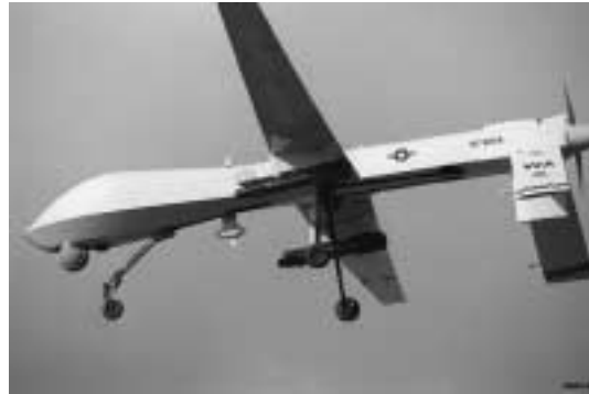
Figure 3. Predator UAV with Hellfire-C
