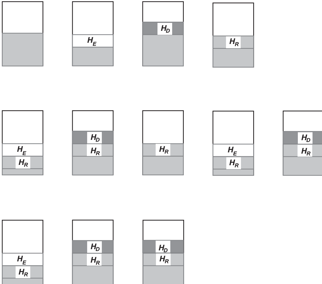
Figure 5. Definitions for entrainment of sediment particles from the sea bed. H_E = thickness of eroded material; H_D = thickness of deposited sediment; H_R = thickness of sediment resuspended, or disturbed, by wave and current action during a specified time interval.
