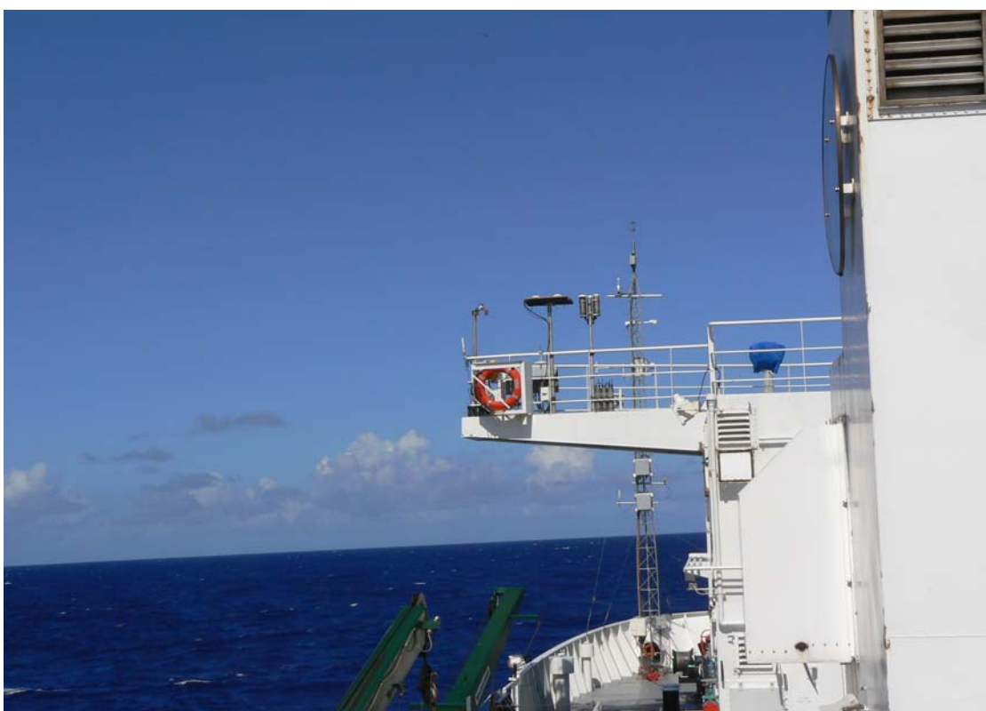
Figure 9-1: PSD instrument tower, partly obscured by the port bridge wing, which holds some of the radiometers deployed for the comparison project.
