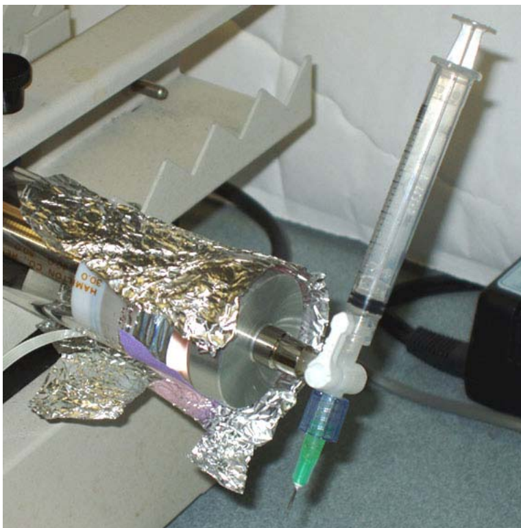
Figure 26. Zero-headspace reactor used for to measure degradation kinetics by iron-activated hydrogen peroxide. Sampling is performed via the syringe.
