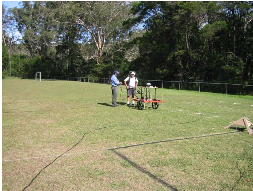
Figure 1-1. Photo of trial with EM63 cart and the gradiometer instrument (right).
