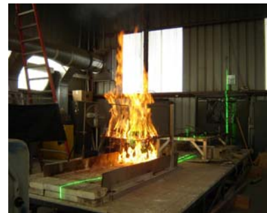
Figure II-4: Riverside Fire Laboratory-Research on transition of surface fires to crown fires.
