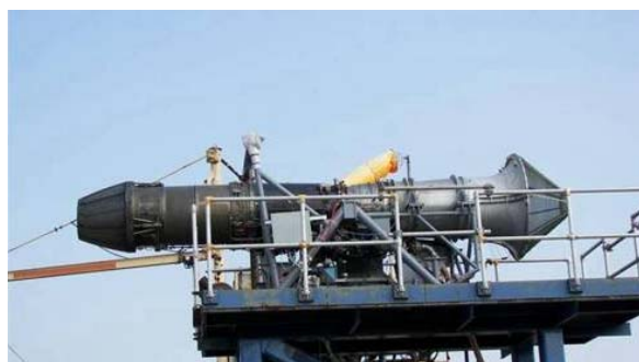
Figure II-5: Measuring the engine noise of an F404 aircraft engine on a test stand.
