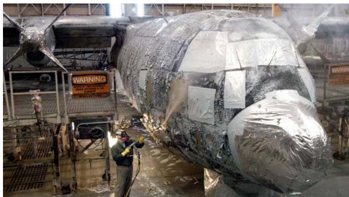
Figure II-17: Studies of the fundamental mechanisms of how methylene chloride and phenolic coatings removers function will help aid the design of environmentally benign alternatives.
