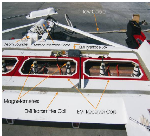
Figure 2-6. The marine sensor platform is shown with the hatch covers removed. Many of the system components are identified.
