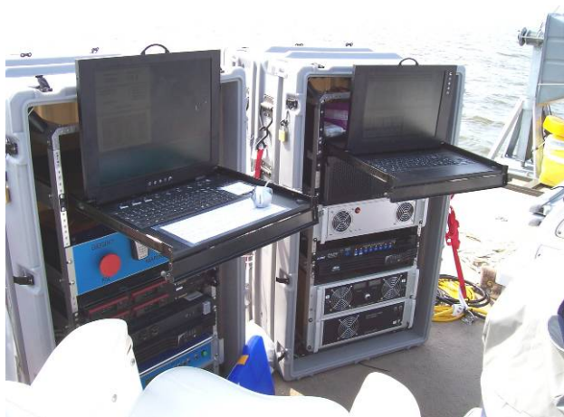
Figure 2-3. All sensor data are recorded by the computers in these data racks mounted across from the drive console, near the port rail.
