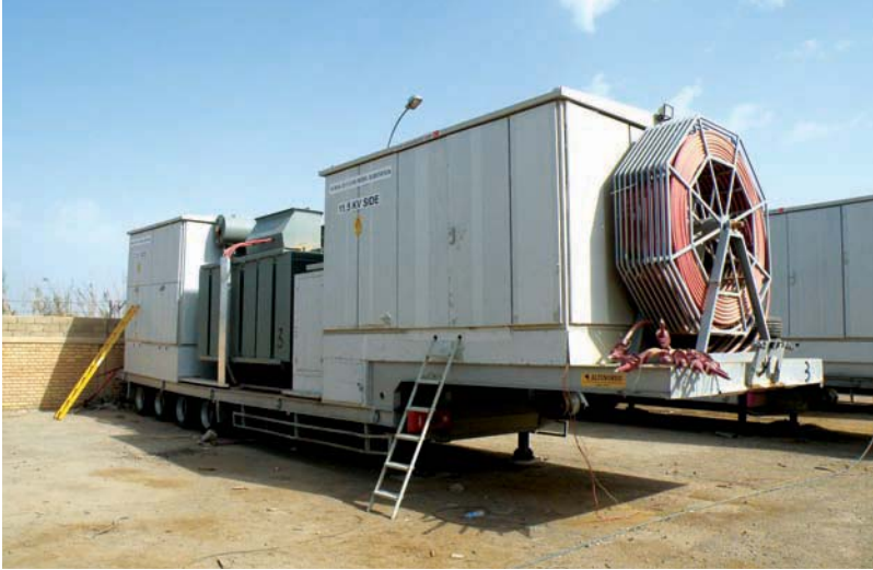
33/11kV Electrical Mobile Substation and exterior condition of trailers at the MOE's Ramadi outdoor warehouse facility.
