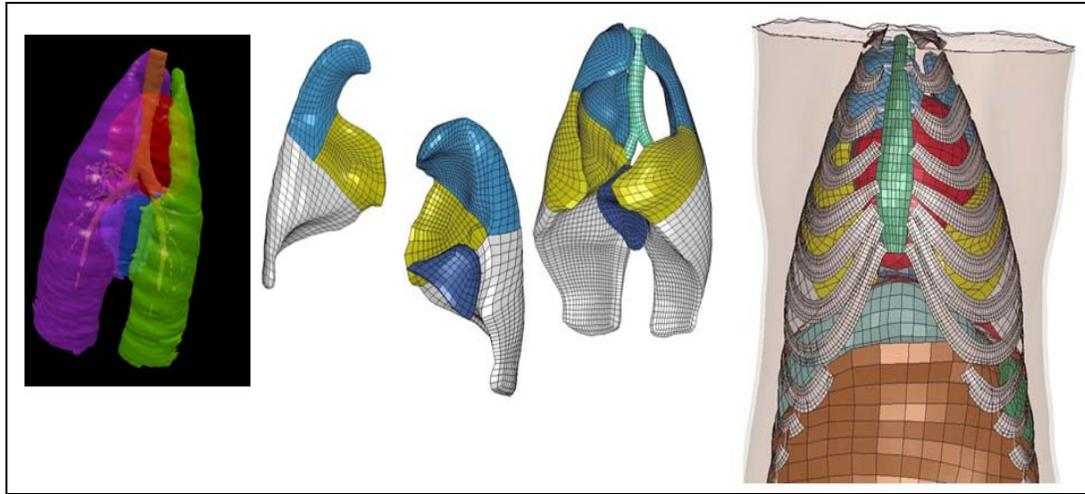
**Figure 50. Detailed finite element model of swine lungs and their incorporation in swine torso.**
