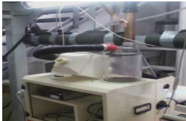
**Figure 11: Aerosol Generator**
