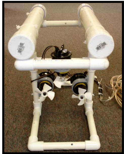
Fig 3 three thrusters give the ROV mobility forward, back, left, right, up & down
