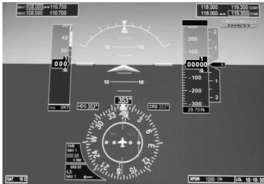
Figure 1. AGARS primary flight display.
