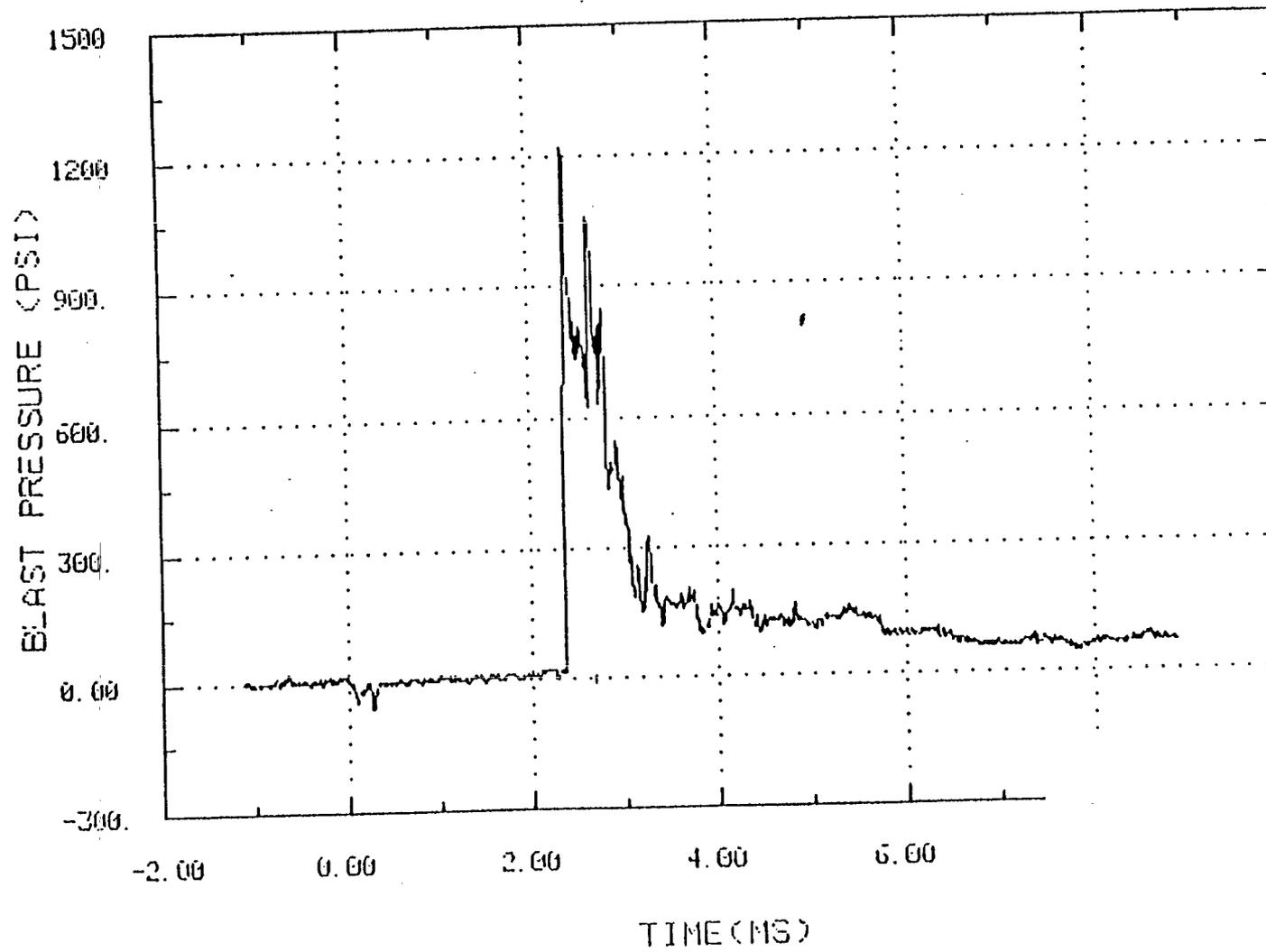
Figure 10. Gas Pressure in the Gravel Gertie Staging Area
