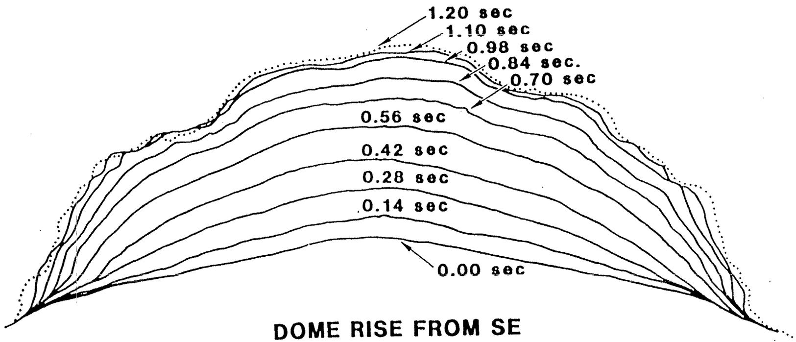
Figure 11. Gravel Bed Profiles during Dome Rise
