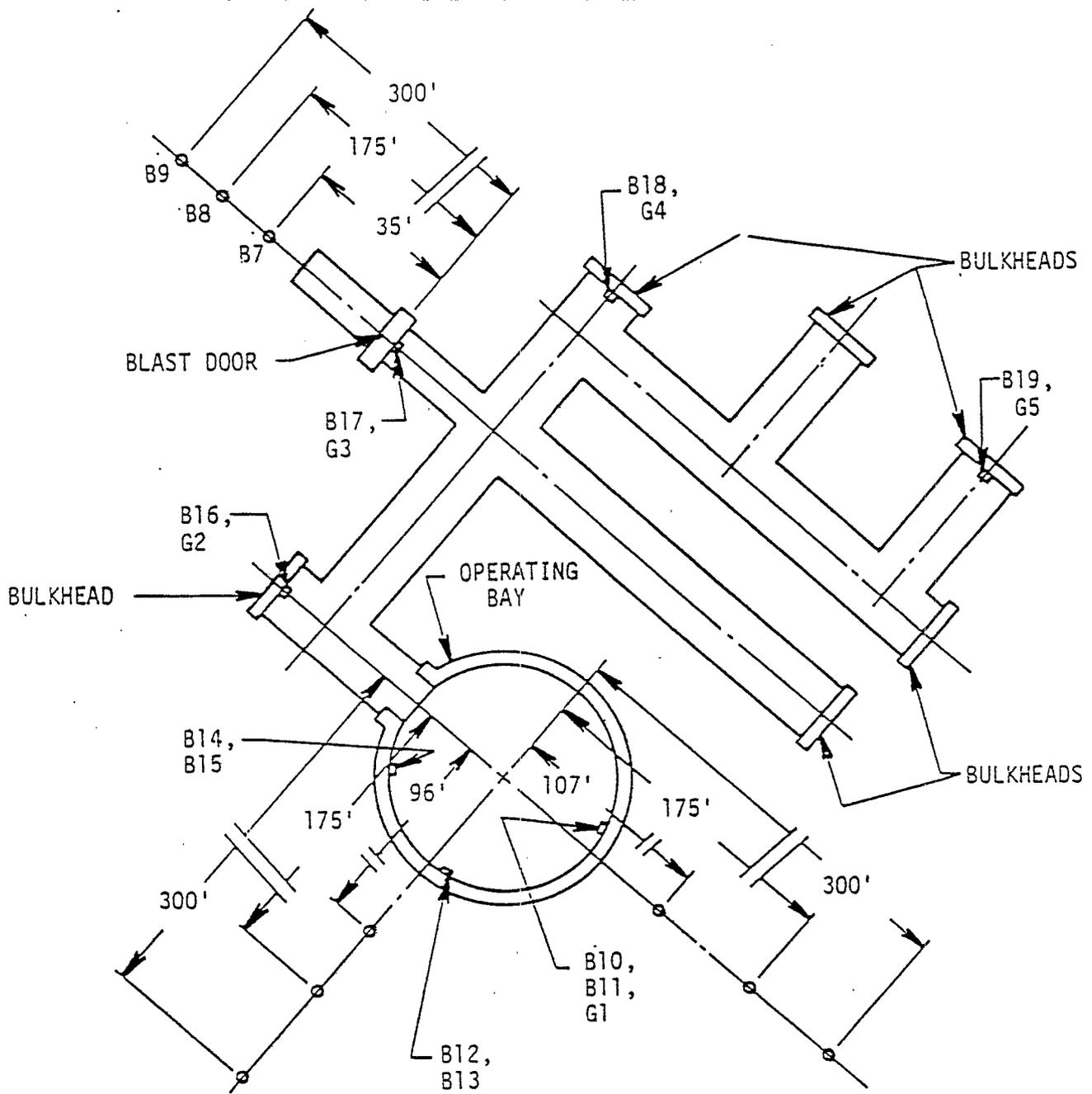
Figure 4. 1962 Gravel Gertie Test Structure with Transducer Locations
