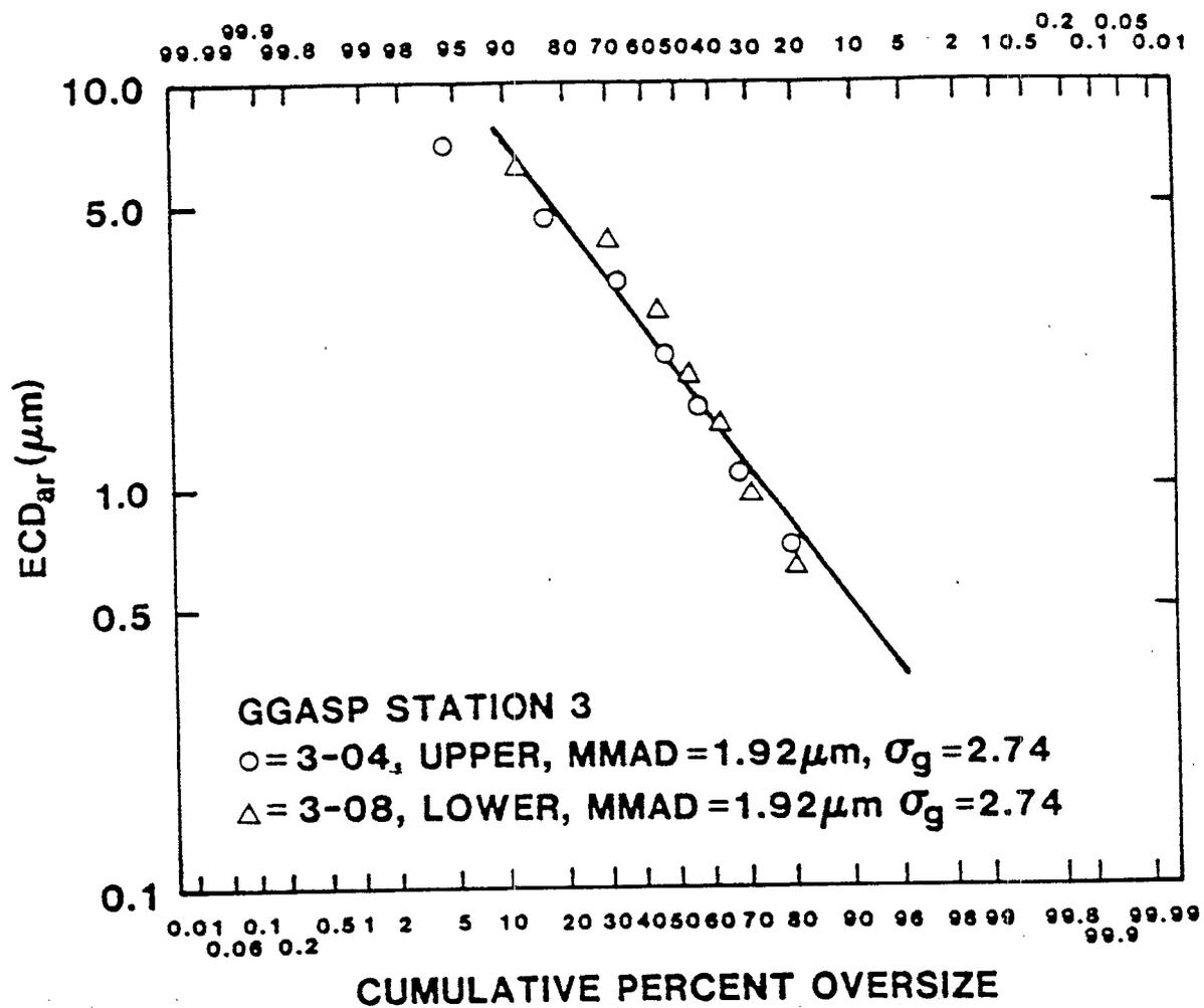
Figure 6. A Log-Normal Fit to Cascade Impactor Data in Round Room Showing Effective Cutoff Diameter as a Function of Cumulative Percent of Mass Oversize
