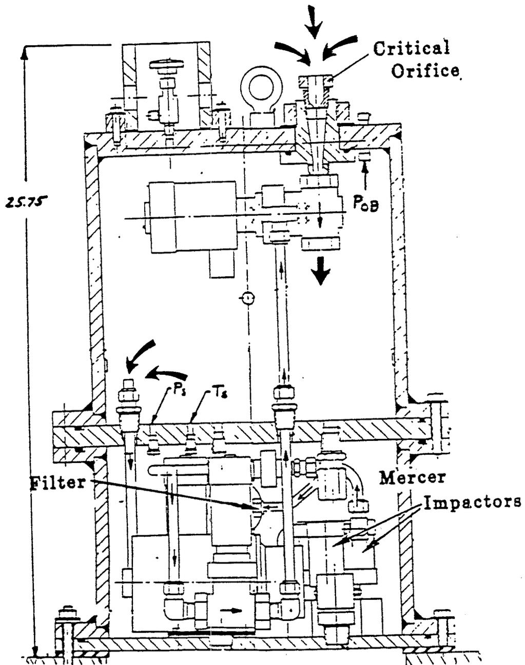
Figure 5. Blast Proof Air Sampler and Cascade Impactor
