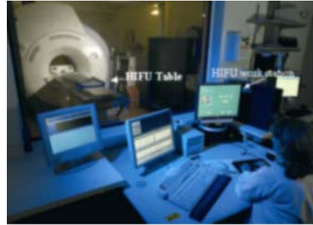
Figure 2. The high intensity focused ultrasound unit with a 1.5 Tesla MR scanner. The workstation is also shown.
