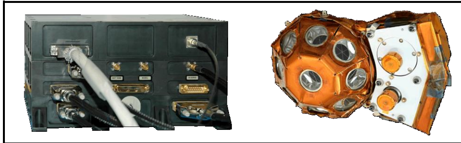
Figure 1. T2L2 Flight Model: The electronic unit (left), and optical units together with the LRA (right).
