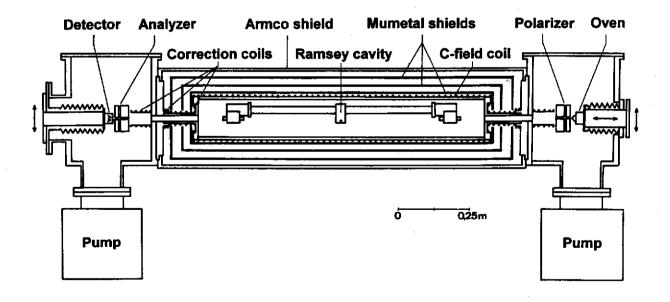
Figure 2. Vertical section through the reconstructed CS1 primary clock.
