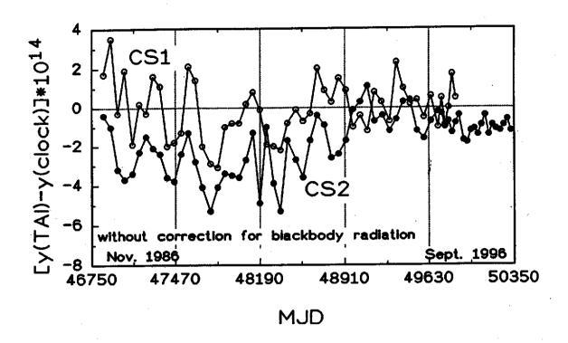
Figure 1. Ten years of frequency comparisons of the primary clocks CS1 and CS2 of the PTB with International Atomic Time, TAI. The data from BIPM Circular T are 60-day averages, the symbols are plotted at the end of each interval. MJD: Modified Julian Date.
