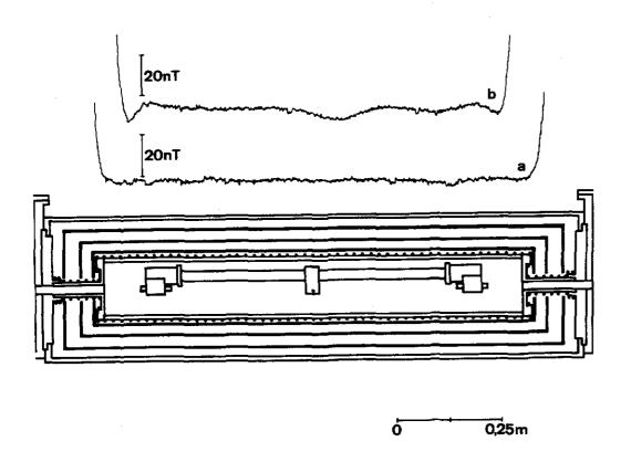
Figure 4. Plots of the axial magnetic field in the beam tube of the CS1. The position of the cavity, the magnetic shields, the solenoid and the trimming coils are shown for clarity; a) residual earth field; b) C-field after final adjustment of the current through the trimming coils, zero suppressed.
