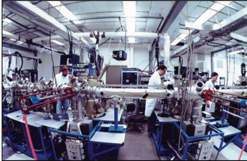
FIGURE 6 The NRL Epicenter includes four MBE systems as well as etching and analysis chambers.
