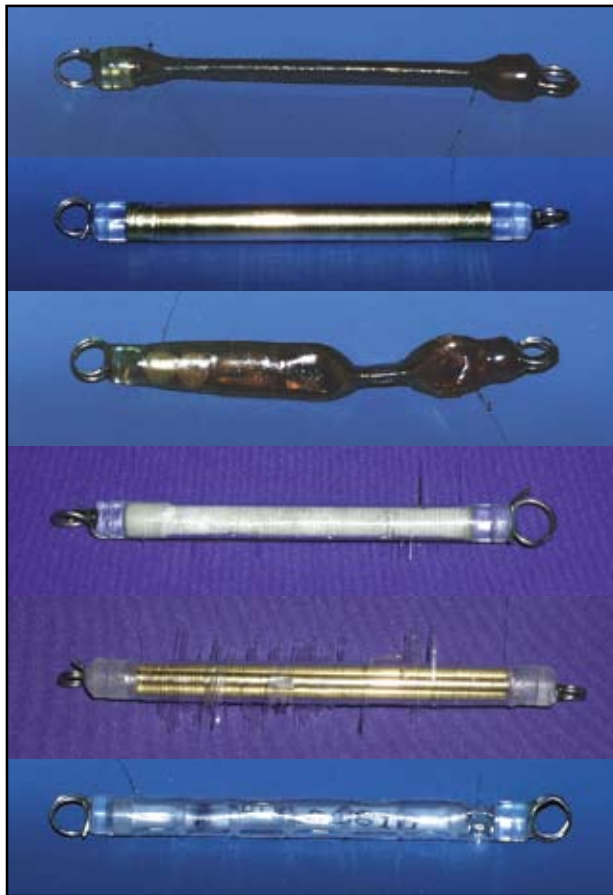
FIGURE 10 Fiber optic hydrophone crush results for six design concepts.
