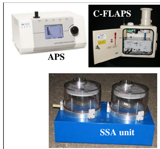
Figure 14: Reference Point Sensors Used during Suffield 07 Trial: Aerodynamic Particle Sizer (APS), C-FLAPS and Slit Samplers (SSA Unit).
