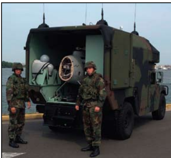
FIGURE 2 The original Dragon Warrior vehicle as it would be transported in a HMMWV along with the onboard Ground Control Station.
