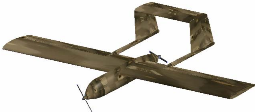
Figure 14: Centerline-thrust hybrid-electric UAS conceptual design
