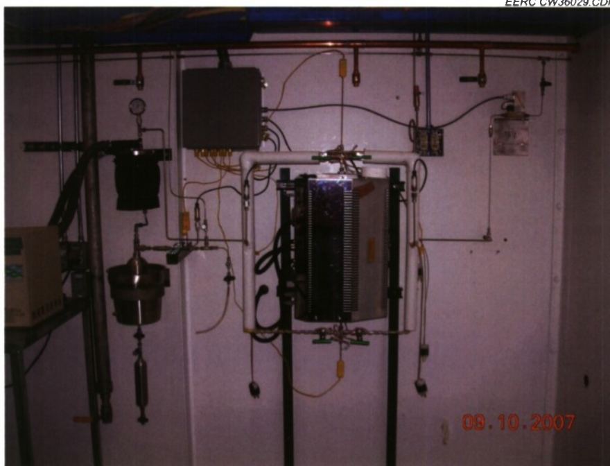
Figure 52. Small continuous reactor system utilized for kinetic rate data experiment.
