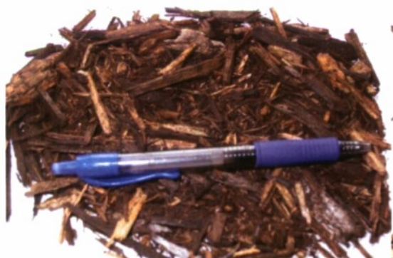
12.5% Moisture Creosote-Treated Railroad Ties
