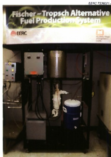
Figure 32. Small-scale FT reactor system for testing small quantities of catalyst with synthetic syngas.
