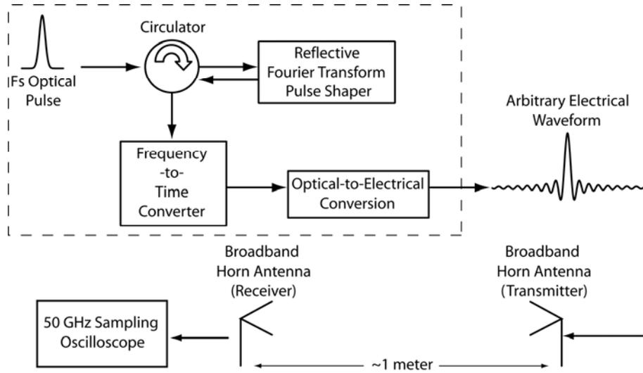
Fig. 10 – Experimental apparatus for broadband antenna phase-compensation experiments.
