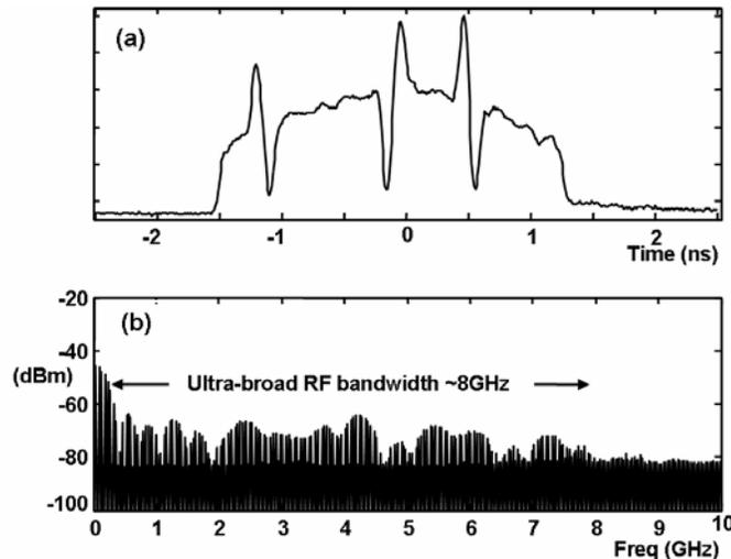
Figure 4 – (a) Monocycle burst waveform. Here, we demonstrate monocycle durations of  $\sim 200$  ps, arbitrary polarity reversals, and variable delay on a scale not achievable via electronic techniques. (b) RF power spectrum exhibiting an  $\sim 8$  GHz bandwidth.
