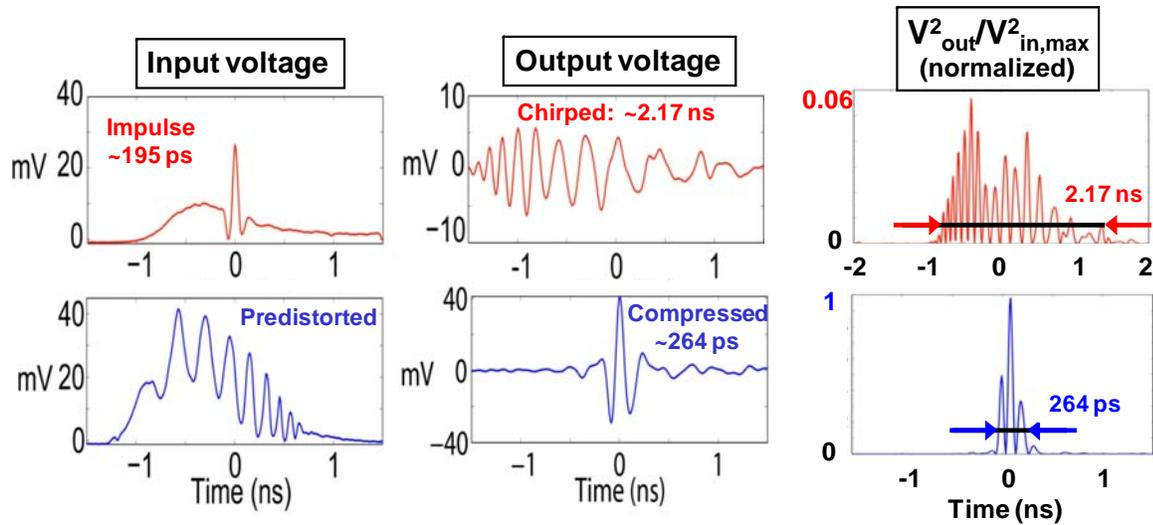
Fig. 17. Experiments with log periodic antenna-horn antenna link. (top row) Experiments with  $\sim 195$  ps impulses. (bottom row) Experiments with time-reversed impulse response used for excitation, resulting in compressed output pulses.
