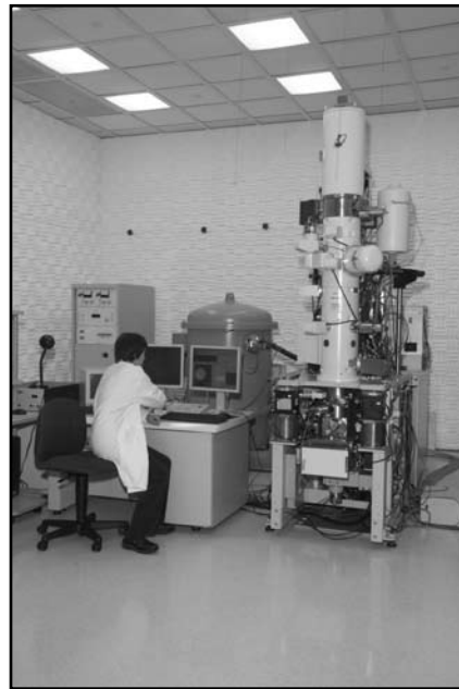
Transmission electron microscope located in one of the NSI's environmentally controlled laboratories.
