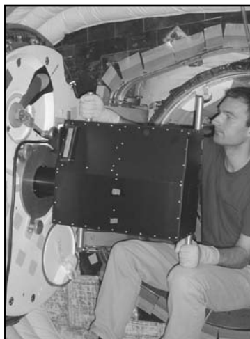
SHIMMER being readied for flight on the Space Shuttle. SHIMMER, a Michelson Interferometer, will map the globe in atmospheric trace compounds.
