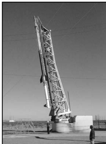
A Black Brant rocket being readied for flight at the White Sands Missile Range. The rocket is carrying NRL's advanced spectrometer for studying stars at soft X-ray wavelengths.
