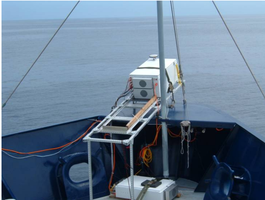
Figure 5. SeaTROLL mounted on the bow of R/V New Horizon during 2005 field test [Fully assembled SeaTROLL system mounted on rails and extended out over bow of ship]
