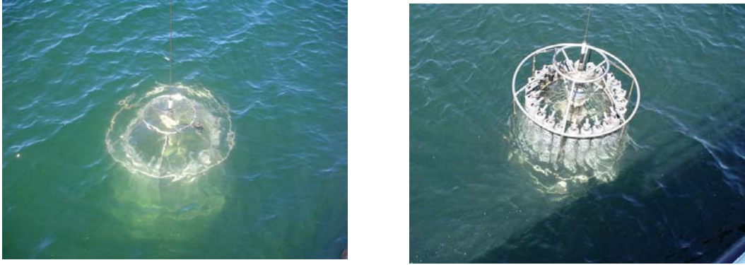
Figure 8. A simple illustration of different water types shown by comparing the details of the R/V Thompson's partially submerged CTD cage. On the left, the more turbid case, the structure of the cage is blurred. On the right, a less turbid case, the bottom ring, while wavy due to the surface, is clearly visible.
