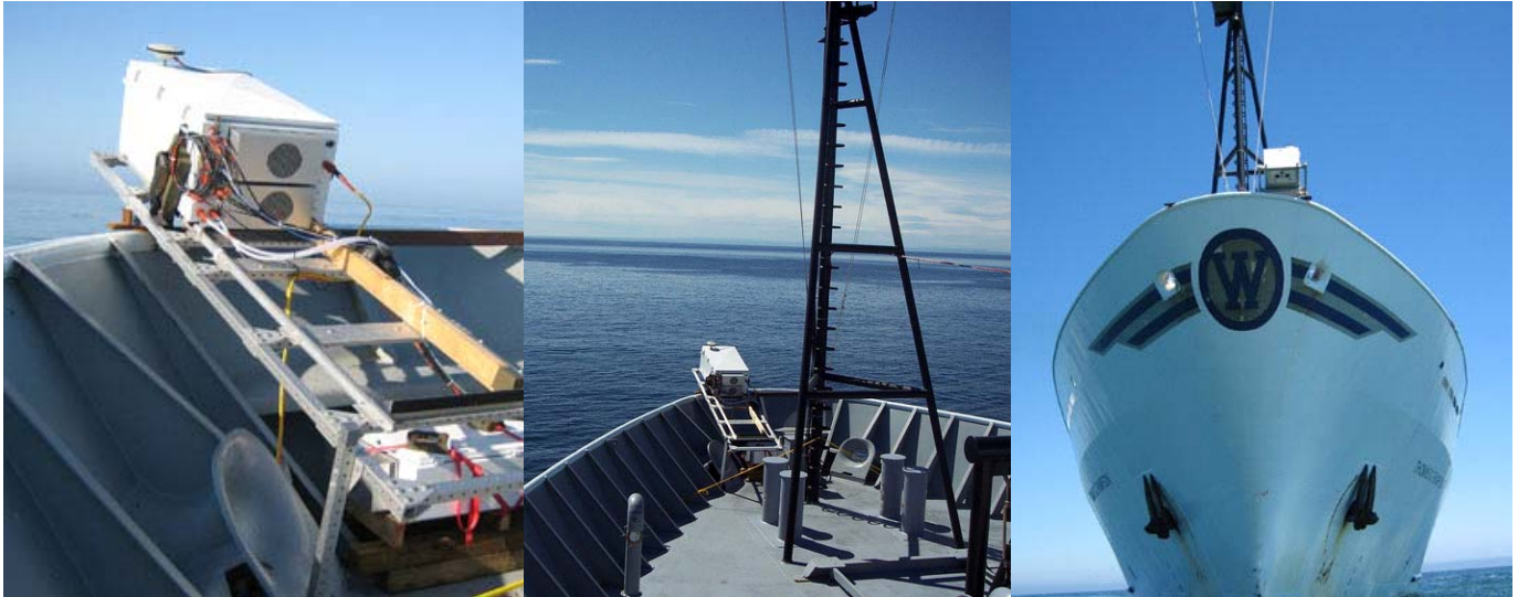
Figure 6. SeaTROLL mounted on the bow of R/V Thomas G. Thomson during 2006 field test [A series of photos show the installed SeaTROLL system. The leftmost photo shows the system mounted on its rails and deployed over the front edge of the bow. The center photo was taken from the bridge, looking towards the bow. The rightmost photo is taken from in front of the ship, looking up from the water. The front half of the system is visible.]
