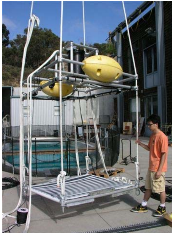
Figure 2. A photograph of the apparatus show in Figure 1b. A camera with floats is on the top of the fixture. Below is a set of four lights and below that is a test target that is printed onto a screen.
