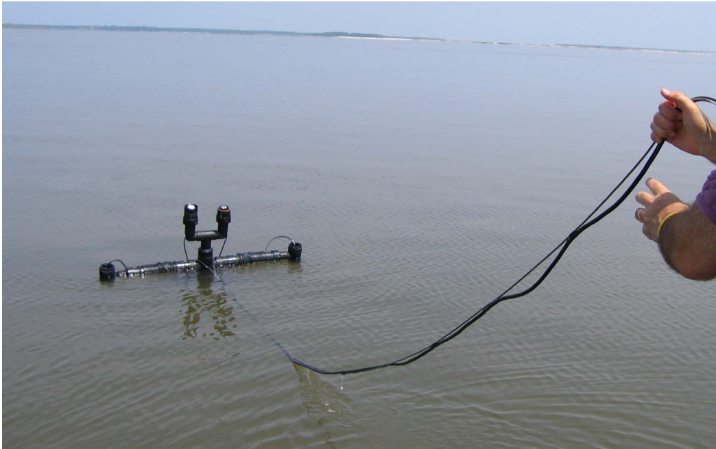
Figure 1. Typical deployment of Satlantic ocean color buoy in dark waters around Sapelo Island [picture of the buoy afloat in still brown water at the end of its conducting Kevlar tether; its above-water reference irradiance sensors ride about 0.5 meter above the air-water interface on a black PVC post and its in-water radiance sensors point down about 5 cm below the water surface at each end of a black PVC spar]
