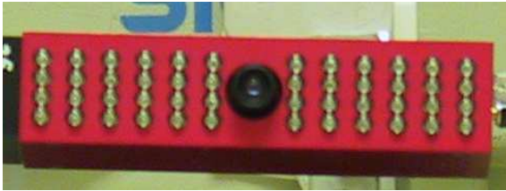
Fig. 1. The TOF 3D range image camera. The camera simultaneously generates intensity images and range information of targets in its field-of-view at a rate of 30 Hz with an active range of 7.5 m.
