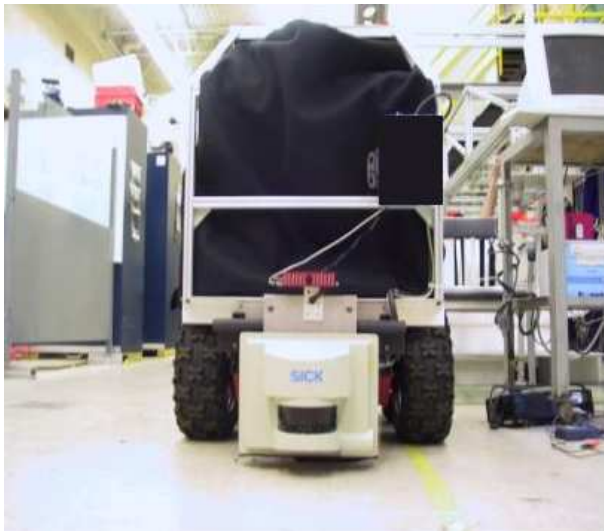
Fig. 5. Experimental setup of the AGV, the scanning laser rangefinder, and the range camera.
