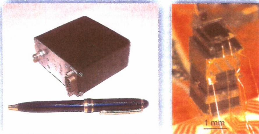
Figure 4. The proverbial black box (left) is a commercial lamp-pumped rubidium clock. On the right is the physics package of a coherent-population-trapping chip-scale atomic clock developed at NIST, which contains the laser, optics, resonance cell with alkali vapor and buffer gas, and photodetector. (Chip-scale clock image from ref. 14.)
