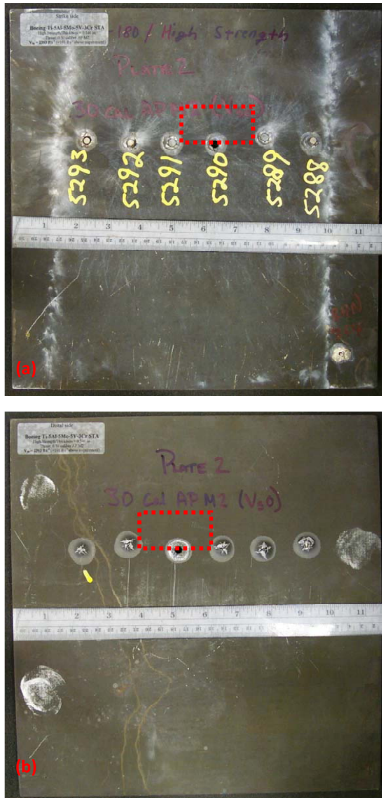
Figure 10. Titanium 5553 high strength plate after V 50 testing against the 0.30-cal. AP M2 threat showing the (a) strike face and (b) the distal side. The red box indicates the area sectioned for examination.
