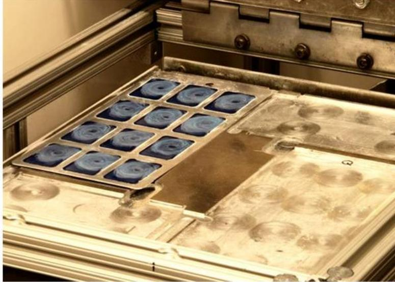
**Figure 3.2.** Close-up view of the high-throughput abrasion testing machine showing a twelve sample array panel loaded in one of four deck positions. *Note the circular abrasion marks on each of the UV-cured epoxy coating samples.*
