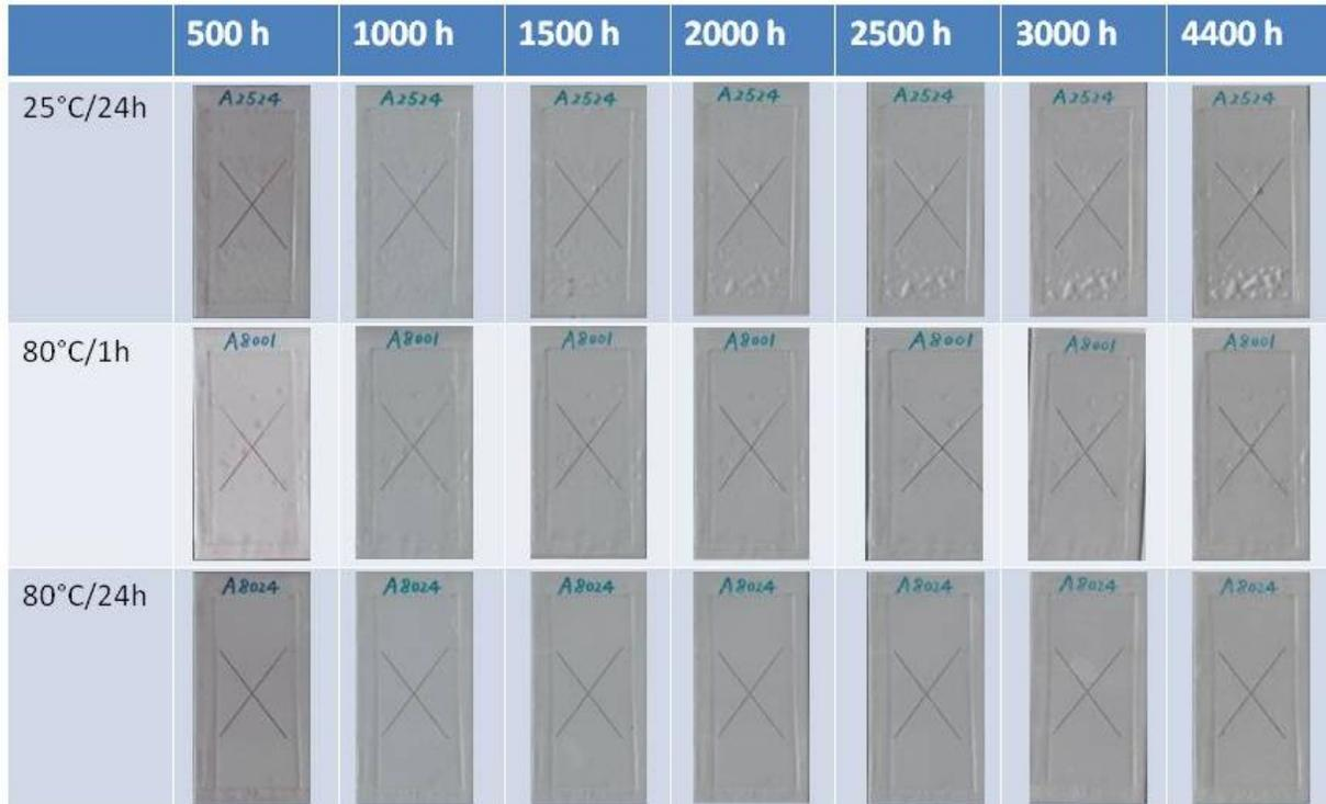
**Figure 3.12.** Images of scribed panels of topcoated samples based on the noTBAF binder system after B117 salt spray exposure. Moving from left to right, salt spray exposure increased. Moving from top to bottom, the amount of thermal energy used to cure the Mg-rich primer increased.
